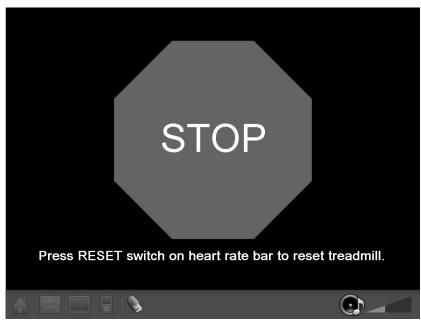
If you see the "Press RESET switch on Heart rate bar to reset treadmill" message in the display, press the reset button located in the heart rate bar.
